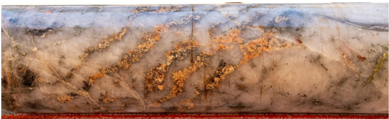
Figure 5 UST textured magmatic quartz body at 495.7m downhole depth 25BRD0037. From within a 0.6m wide interval visually estimated to contain 1% chalcopyrite (0.35% Cu*). Core diameter 61mm.
