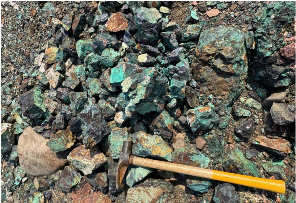
Figure 4 - Example of massive sulphide at the northern trench at the Copper Lamb Prospect (>90% Bornite, <5% chalcopyrite, 1-5% quartz-calcite). Photo taken at NAD83/UTM Zone 11N 505699 E, 7501746 N.
