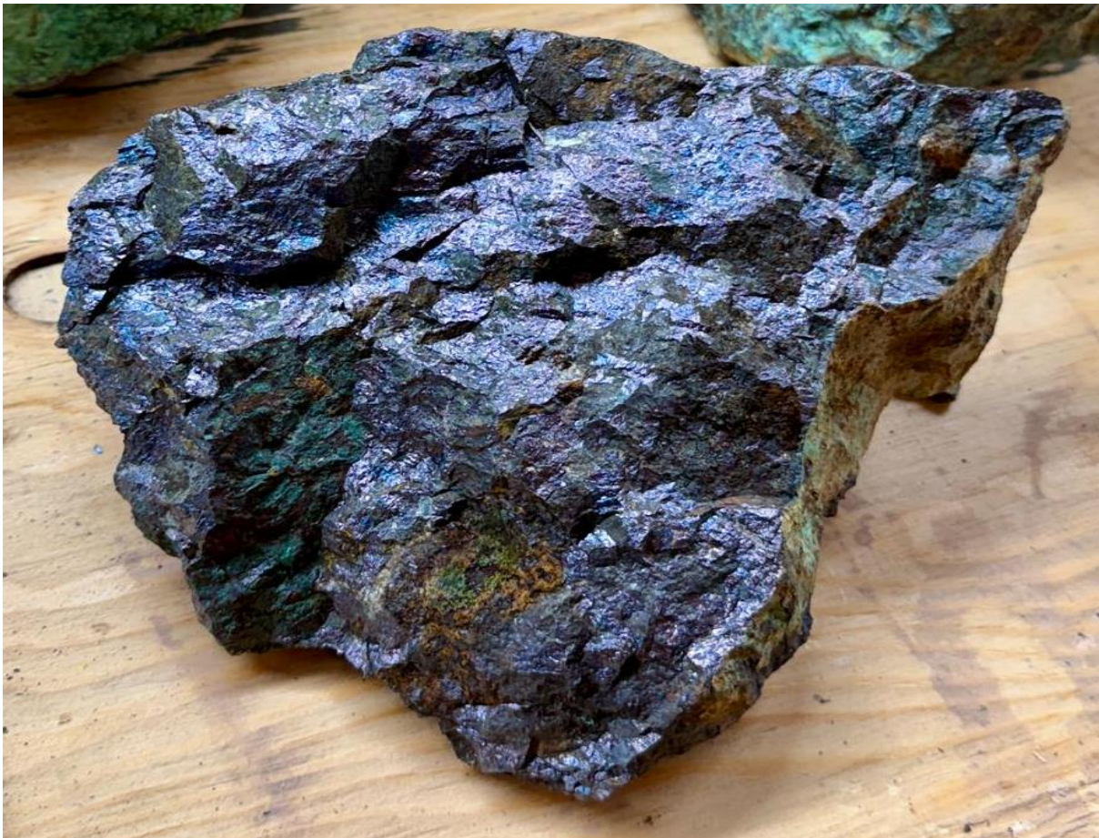
Figure 1 - Example of massive bornite from the northern trench at the Copper Lamb showing. Rock is composed of >95% bornite with 1-3% chalcopyrite and accessory quartz-calcite. Sample is approximately 20cm across. Sample taken from NAD83/UTM Zone 11N 505699 E, 7501746 N.
