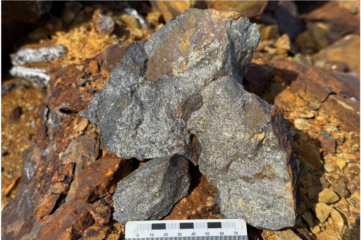
Figure 4: | Rock sample M209549 from Skyfall, a massive sulphide consisting of sphalerite and chalcopyrite. Sample returned results of 13.45% Zn and 0.78% Cu.
