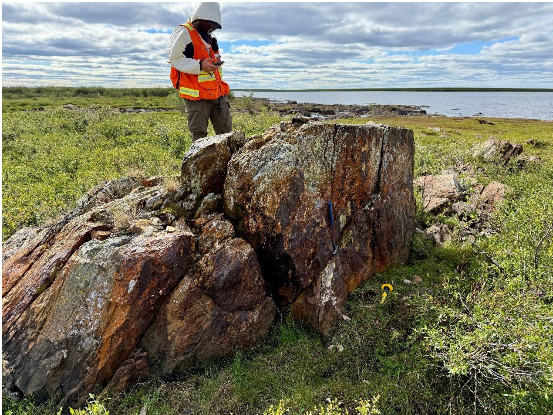
Figure 5: | Outcrop of rock sample M209541, a stringer zone of sphalerite and chalcopyrite at the Spectre VMS showing.
