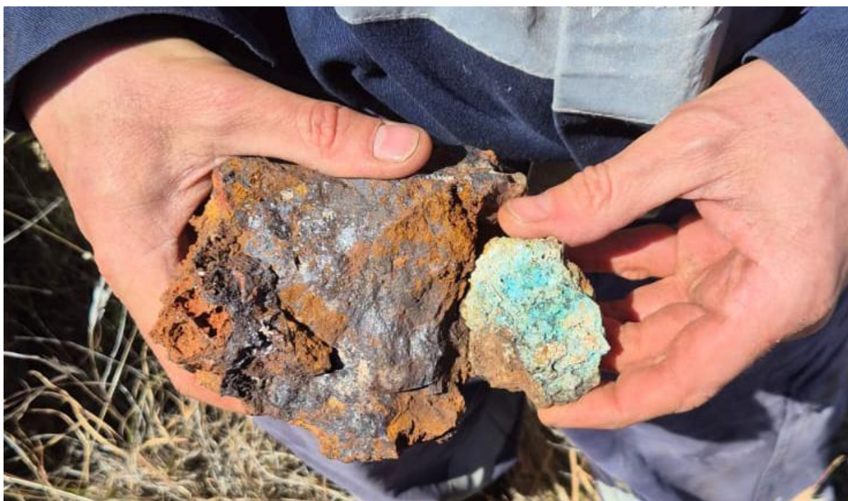
Figure 3. Gossan outcrop (482389E, 7438704N, Sample RK0072) showing classic ex-sulphide boxwork texture identified at VT1 immediately along strike from outcropping Oonagalabi Formation marble with oxidised copper mineralisation present. See Appendix 1 for laboratory assay results. 2
