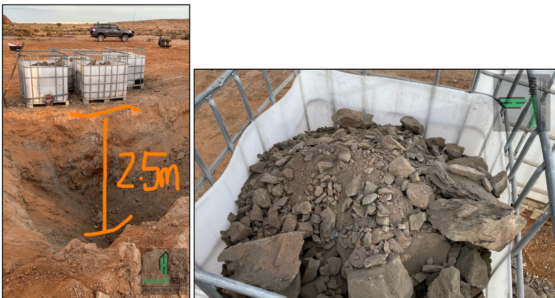
Figure 5: RCFO23015 drillhole sump and an example of the sample recovered
