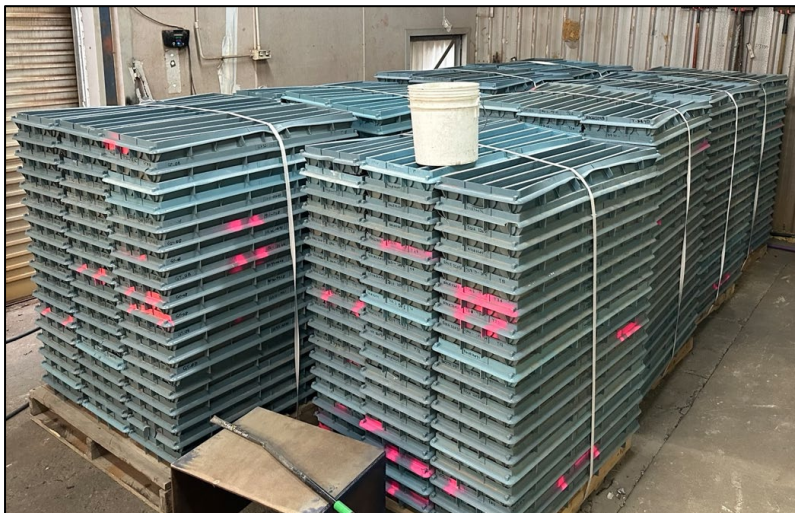
Figure 4: Pallets of trays of \frac{3}{4} HQ3 diamond drill core to be used for testing at ALS Perth
