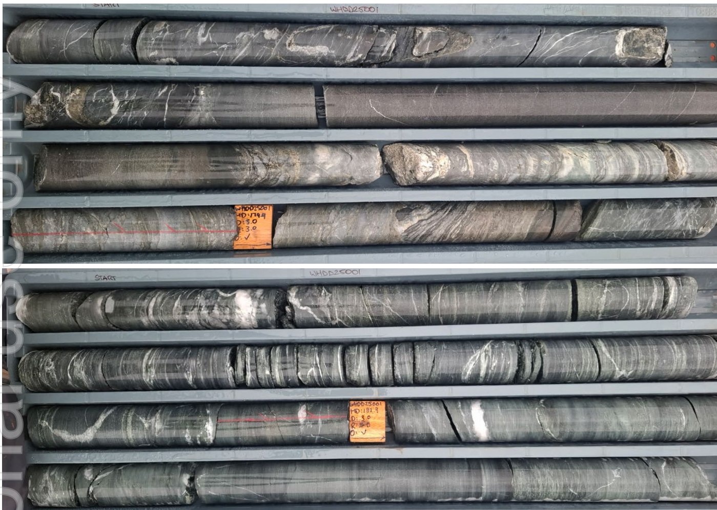
Photo 2. WHDD25001 - ~178-182m Sheared altered BIF with veining and sulphides at Waihi.
