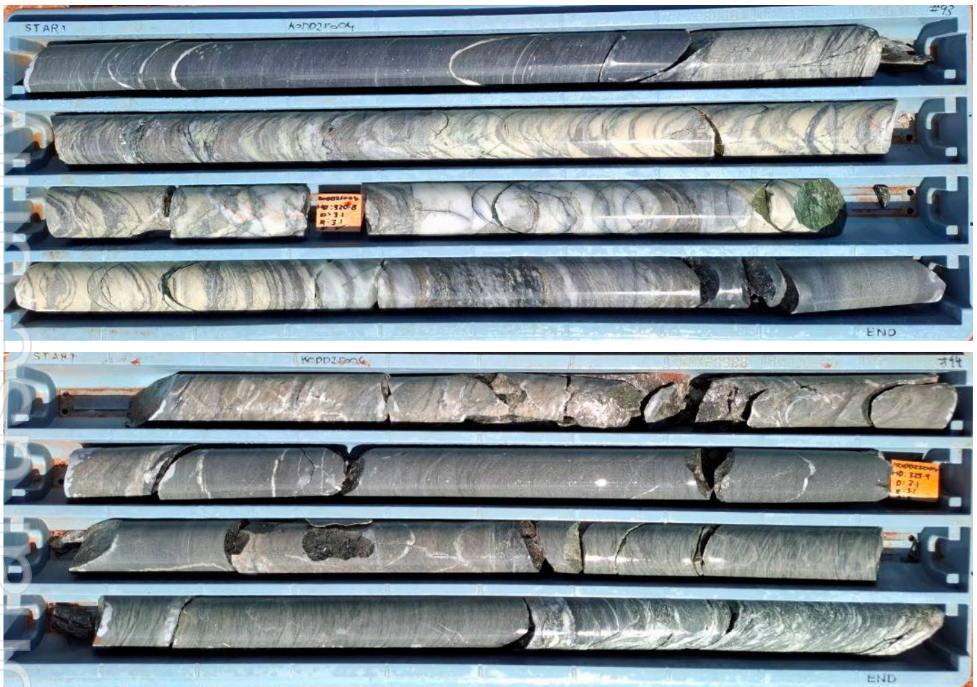
Photo 1. KODD25004 - ~319-323m Sheared altered BIF with veining and sulphides at Korong.
