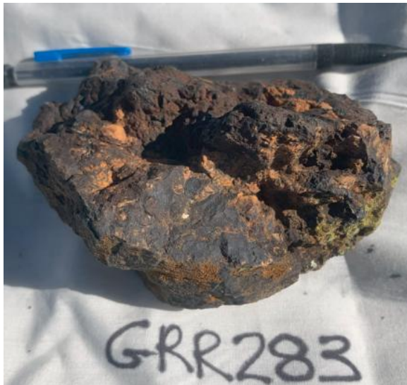
Figure 3: High-grade massive black manganese oxide mineralisation, 33.5% Mn, Sample GRR283
