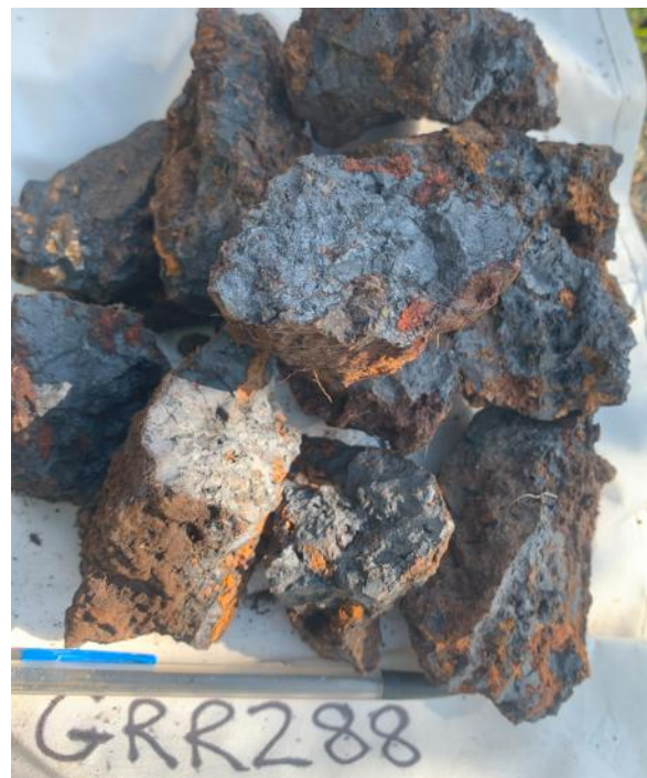
Figure 11: High-grade massive black manganese oxide mineralisation, 36.8% Mn, Sample GRR288
