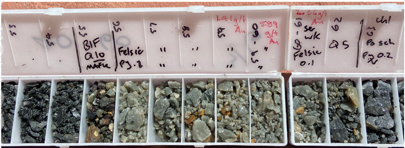
MGTDH002: 3m @ 3.2g/t Au from 59m (including 1m @ 5.9g/t Au) in silica/sericite/pyrite-altered felsic porphyry adjacent to BIF and quartz veining at a sheared basalt contact.
