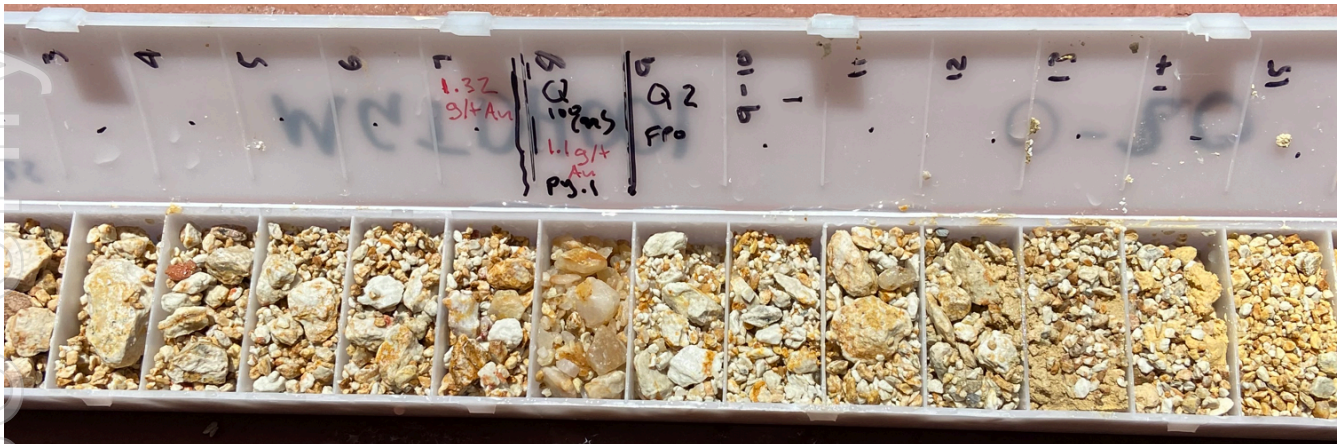
MGTDH001: 2m @ 1.2g/t Au from 7m in weathered and foliated felsic porphyry and quartz veining.
