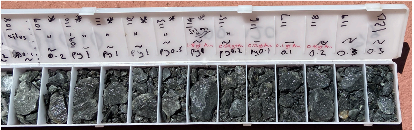
MGTDH010: 5m @ 0.7g/t Au from 114m (including 1m @ 1.8g/t Au) in silica/pyrite-altered, foliated felsic porphyry
