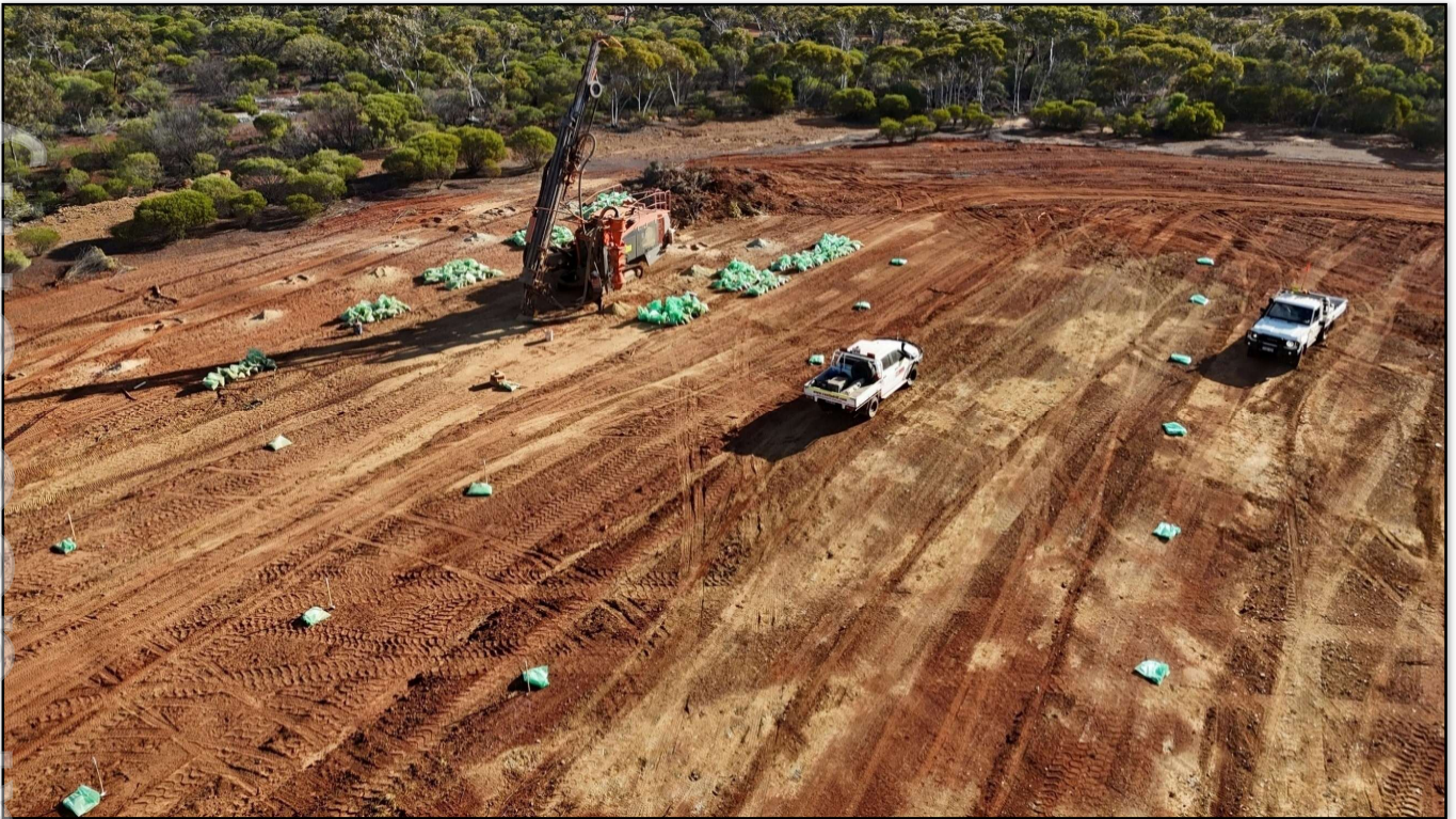
Figure 2: RC drilling in progress at Mt Dimer Taipan
