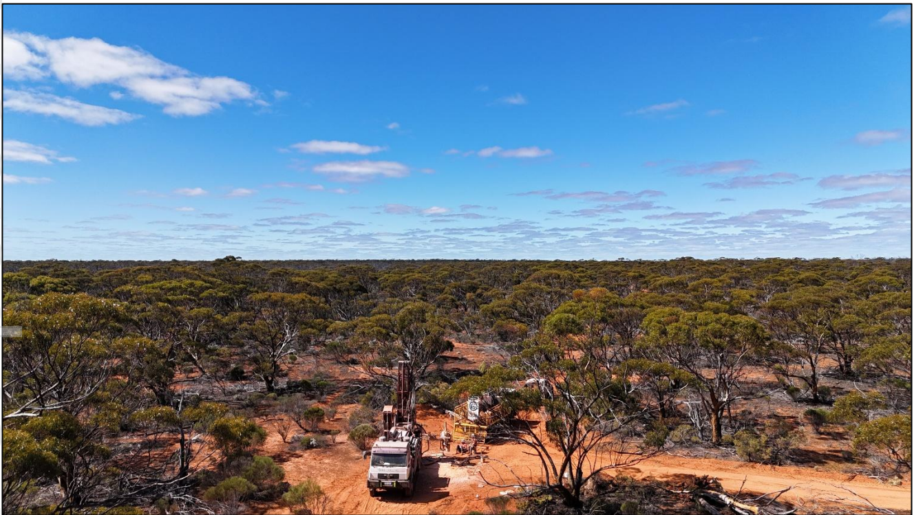
Figure 1: Aircore drilling during the campaign at the Themis South Prospect
