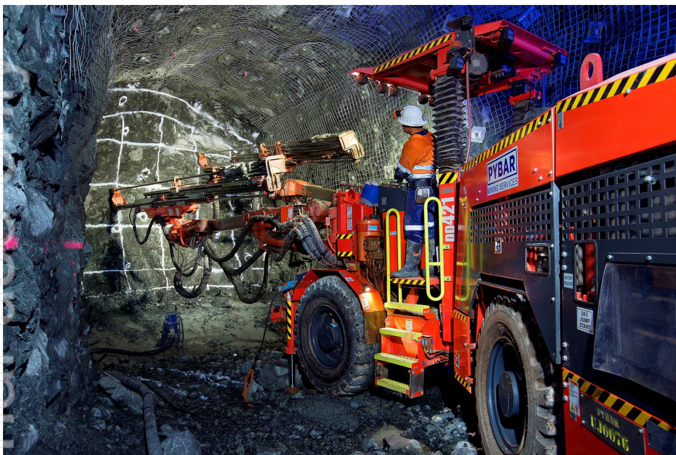
Figure 1 PYBAR jumbo operating underground
