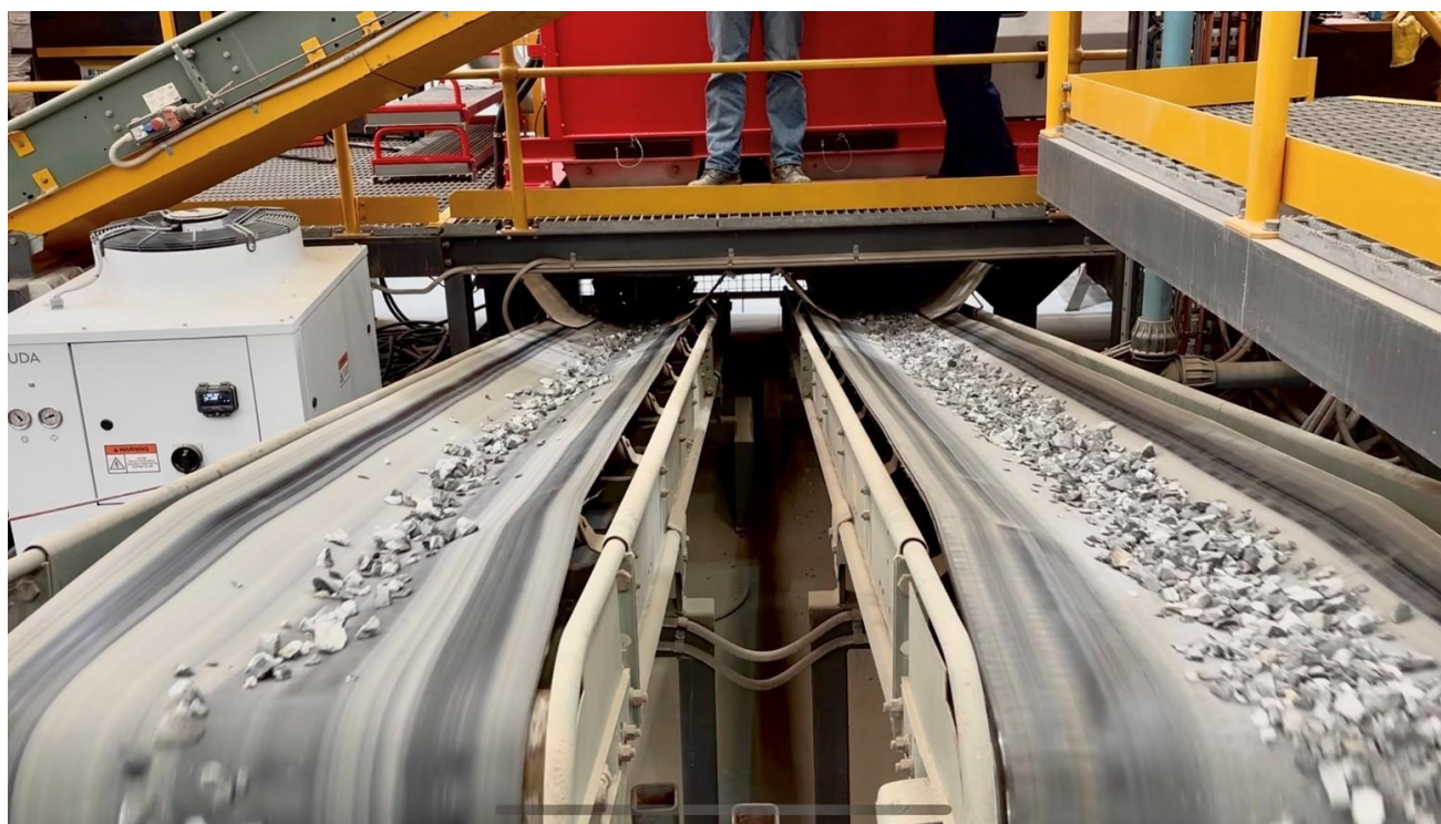
Figure 1. Ore Sorting Tests at the TOMRA Facility processing the tungsten ore from the Cleveland Project, product on the left, waste on the right.
