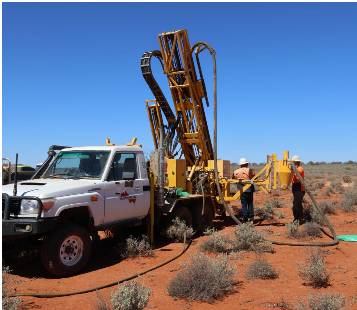
Figure 4: Landcruiser mounted AC Drilling underway at Ariadne-Company Well prospect areas, Minos Gold Project.
