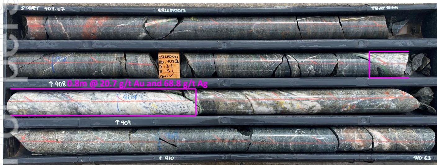
Figure 1: Minos diamond core from 408.7m to 409.5m showing high-grade gold mineralisation in strong quartz carbonate veining (25LLRD013).
