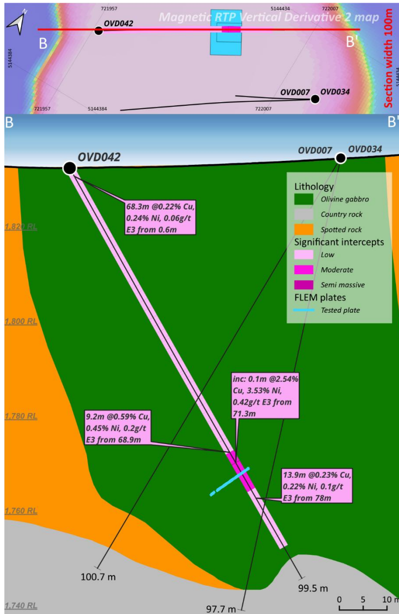
Figure 4. OVD042 cross section
