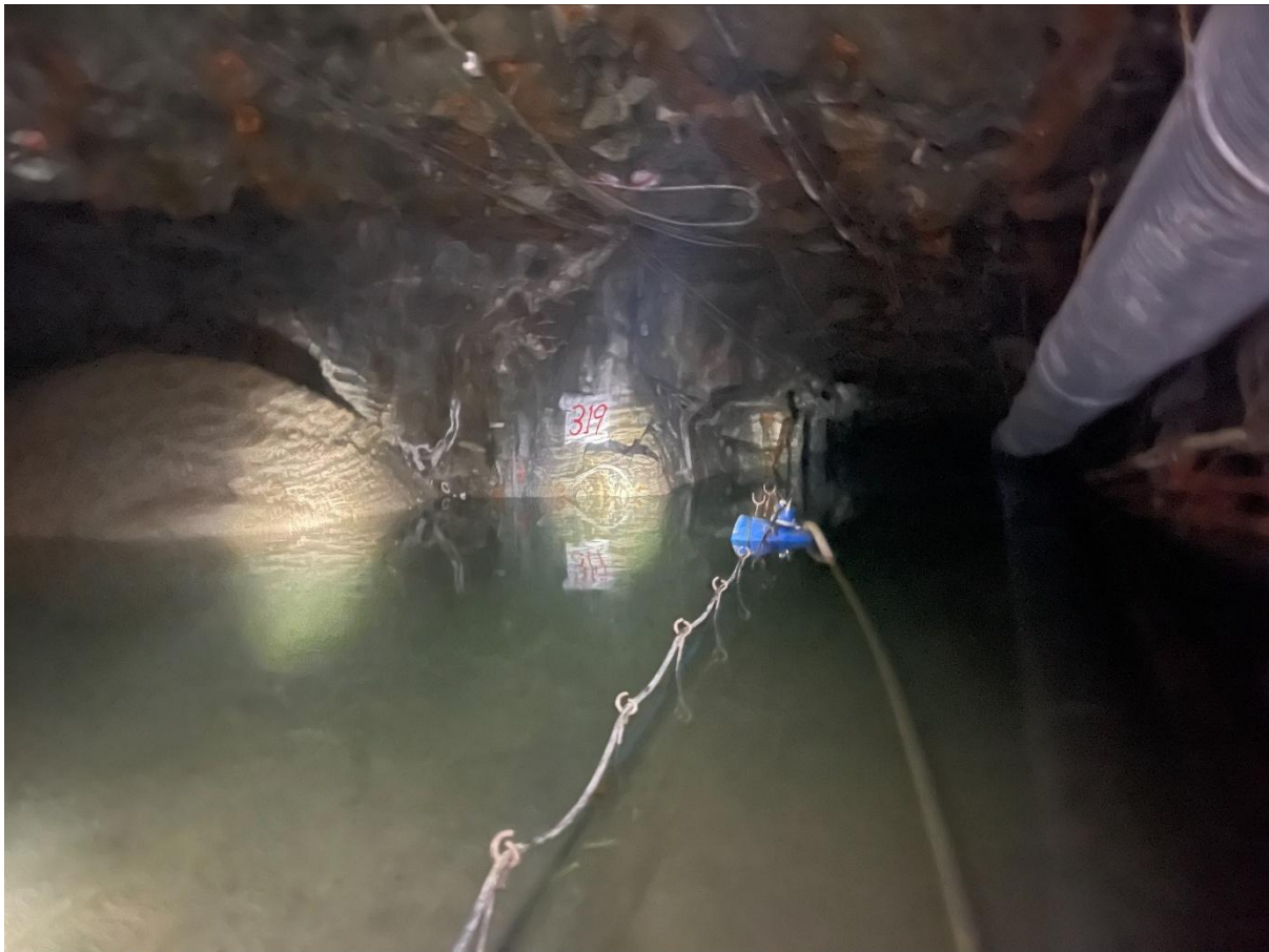
Figure 2: Dewatering activities continue down Stringbean Alley Decline. XC3 (the site of the first planned drilling, reached over the weekend) ore stockpiled to the side (dated 8 th November 2025).
