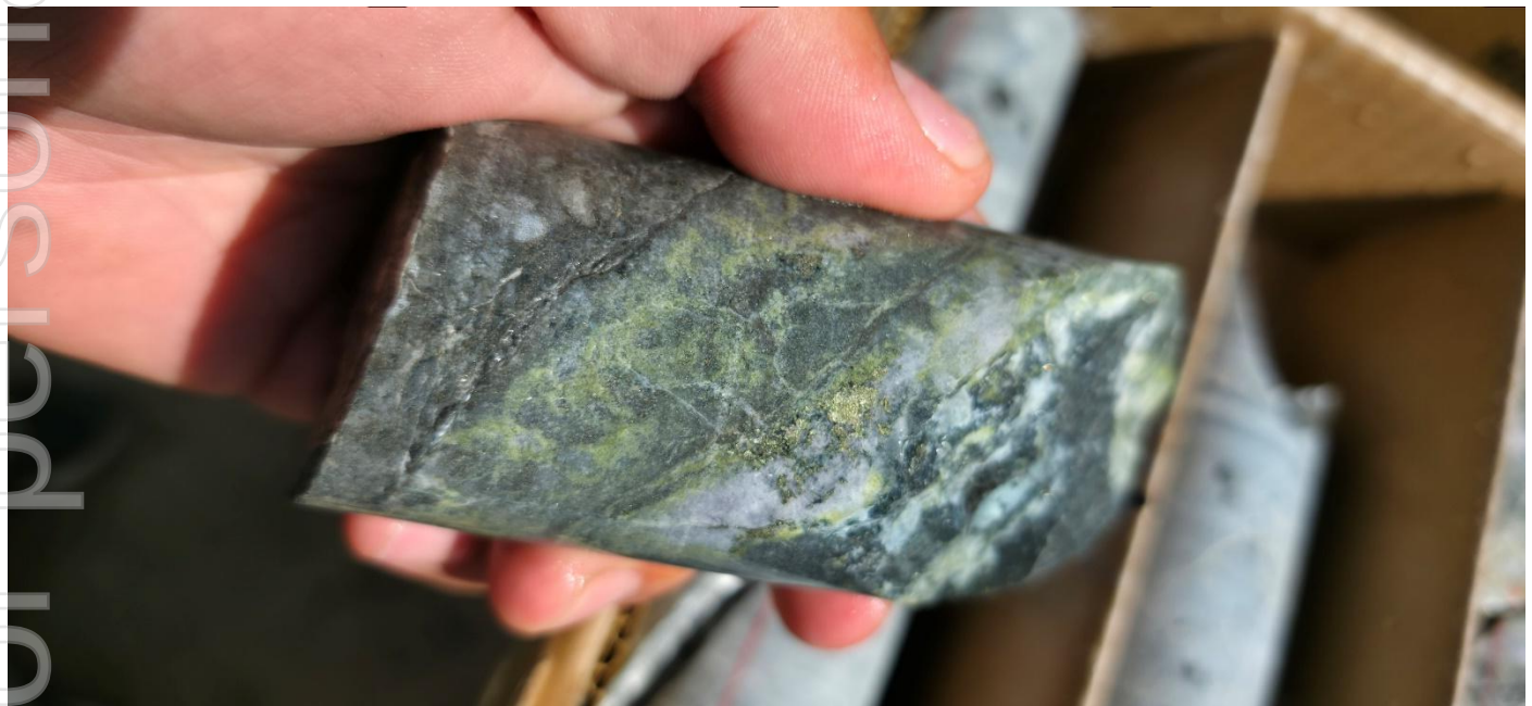
Photo 1. Anhydrite vein with chalcopyrite within altered porphyry from 1162.3m downhole* (refer to Appendix 1).
