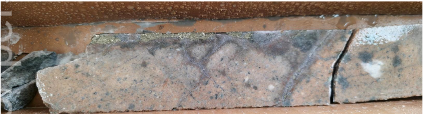
Photo 3. Potassic alteration in 25LLDD0070 from 840m downhole*.
