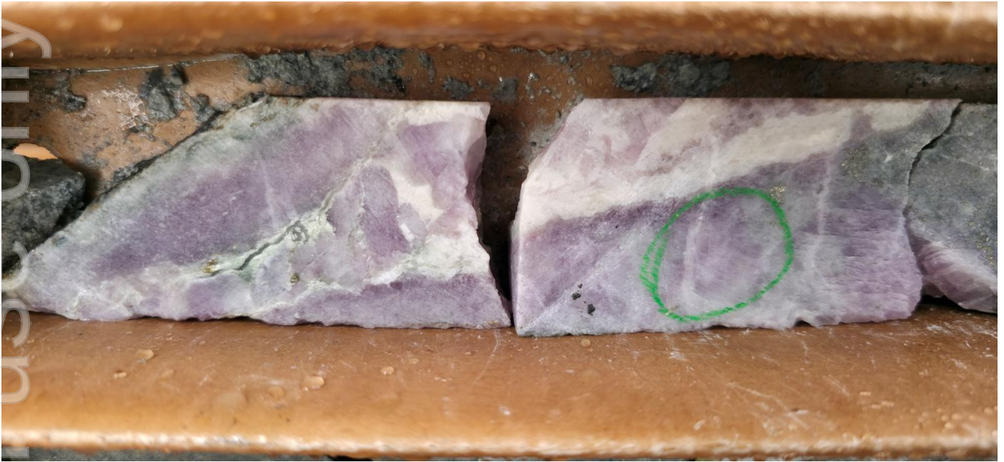
Photo 2. Example of an anhydrite vein with quartz and pyrite from 826.8m downhole*.
