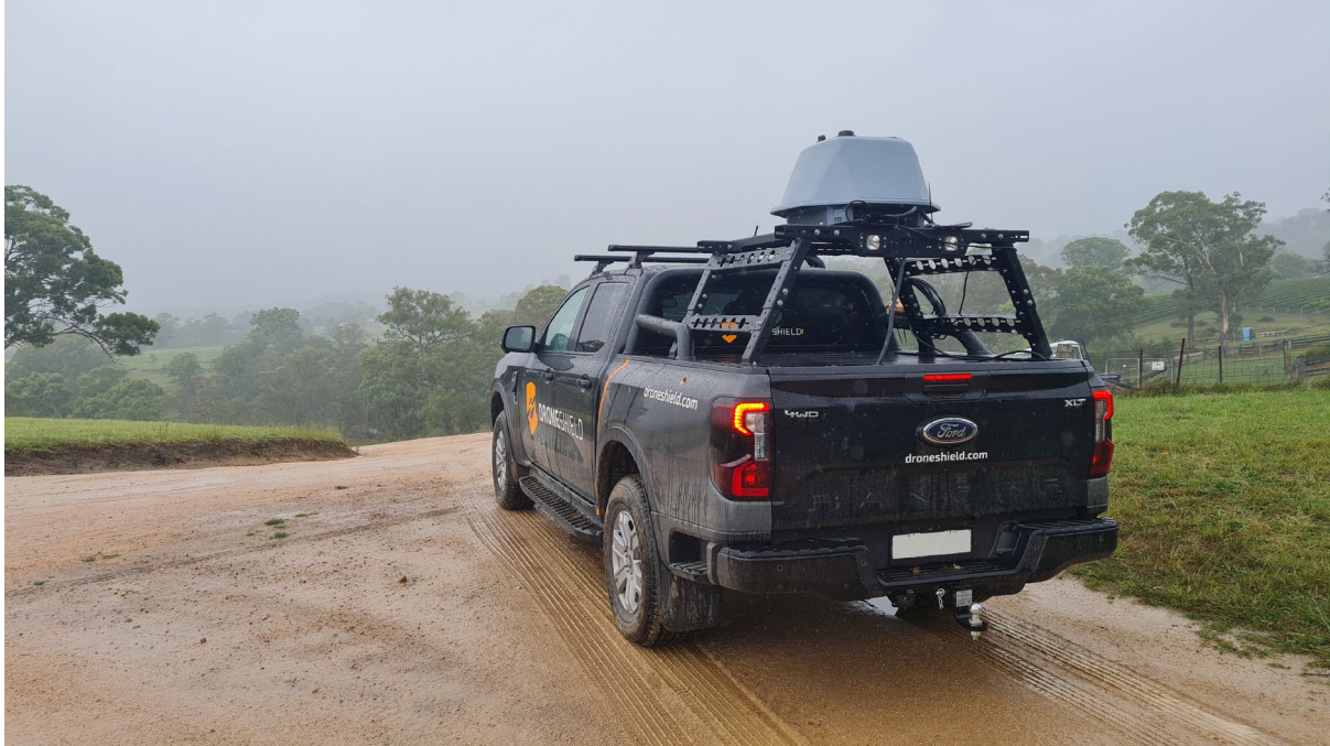
Image: DroneShield DroneSentry-X detect and defeat system
