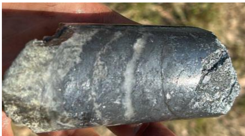
Figure 1: Stibnite and quartz veining from 42.0-42.1m downhole in Dart Mining's first drill hole at Coonambula (CBADD001) part of an intersection of 0.65m @ 32.20% Sb + 2.91 g/t Au + 10.50 g/t Ag from 42.0m.
