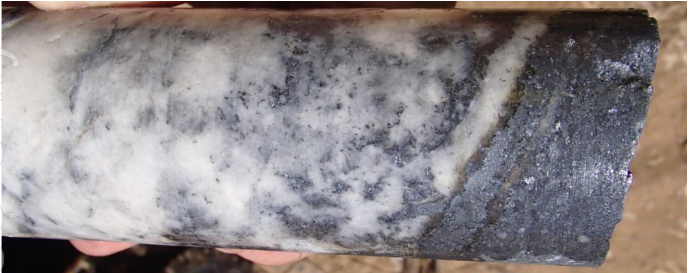
Figure 6: NQ drill core from 131.45m depth from Dart's third hole CBADD003. Massive stibnite on the right of the core from 131.6m, with quartz and stibnite to the left. Detailed logging and sampling are underway, assays expected in December.
