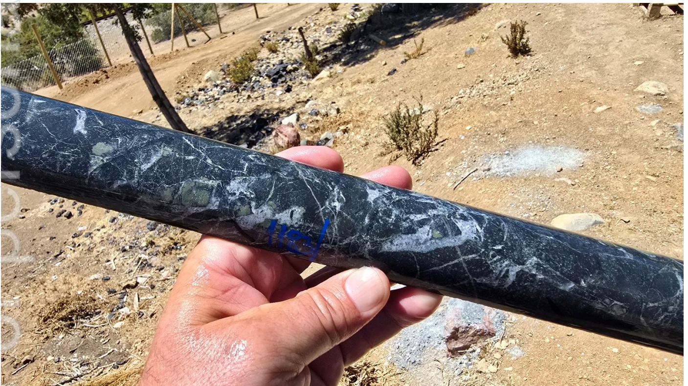
Photo 4. Interpreted crackle breccia from 1183m downhole, which starts from approximately 1160m downhole and continues to the current depth of the hole.
