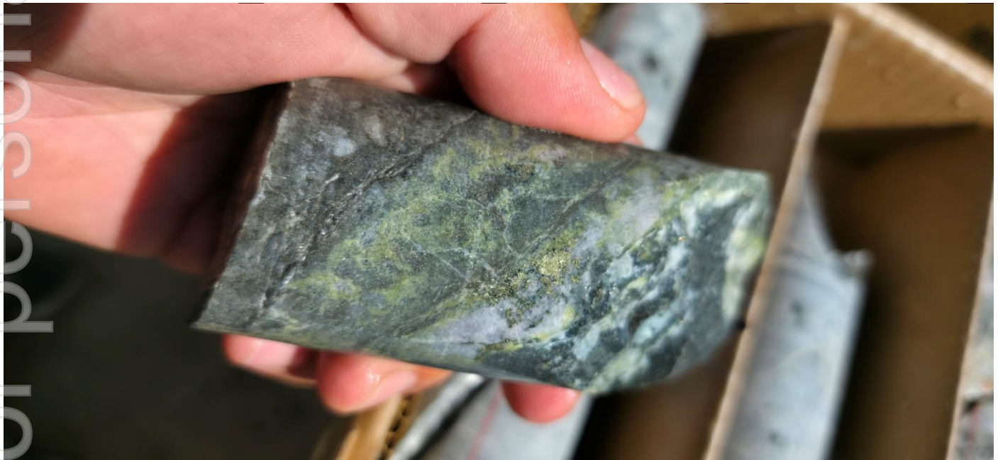
Photo 1. Anhydrite vein with chalcopyrite within altered porphyry from 1162.3m downhole* (refer to Appendix 1).
