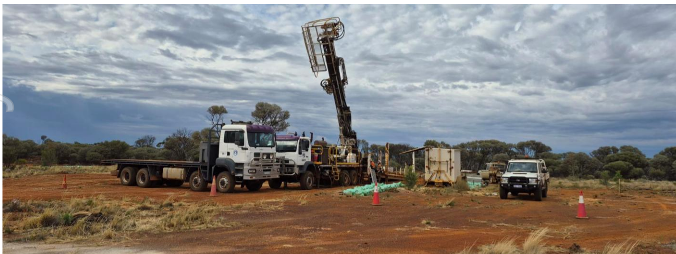
Figure 1: Diamond drilling James Stage 1 metallurgical testwork hole
