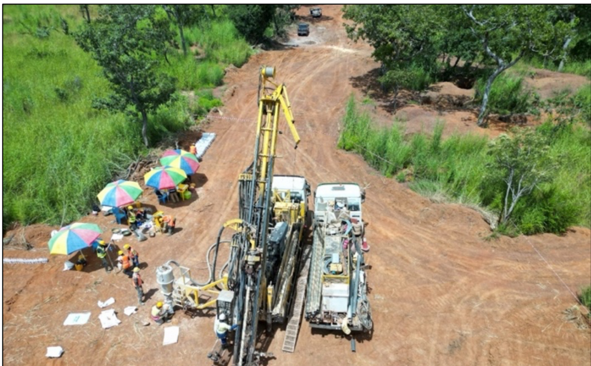
Figure 1 – RC drilling at the Tolé Gold Project, Guinea
