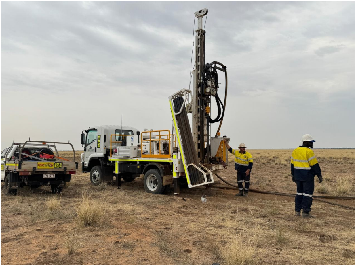
Figure 2 – Aircore drill rig on the first hole of the program
