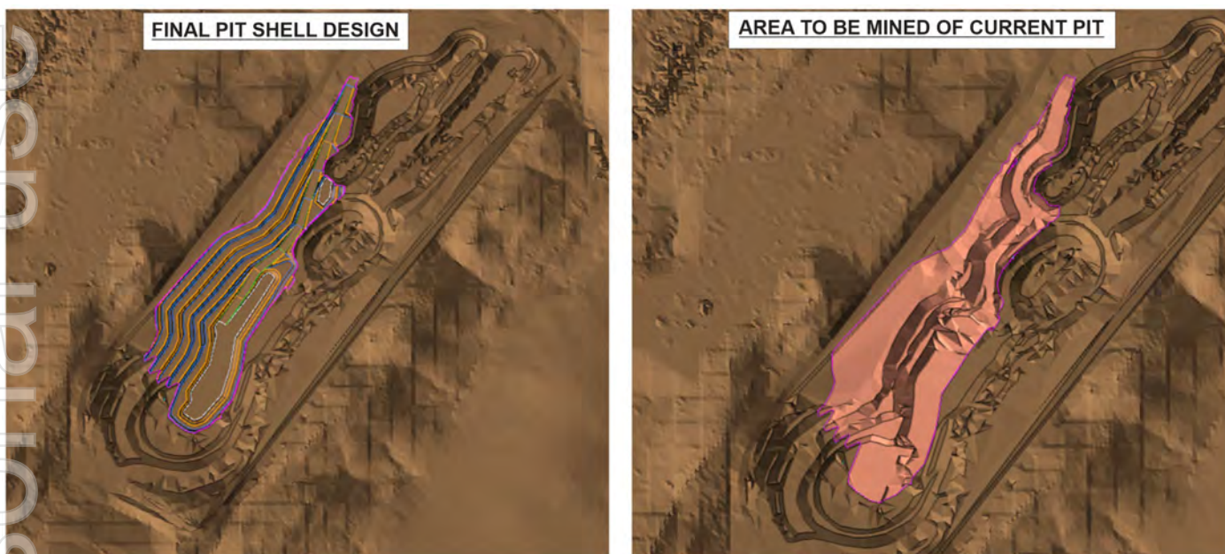
Figure 5.2 - Butchers Creek Open Pit Design
