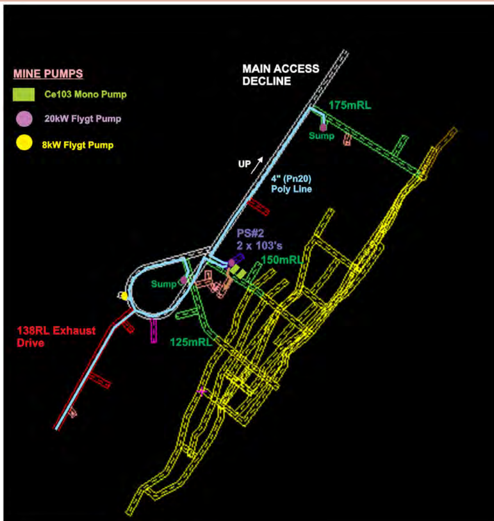
Figure 7.10 - Plan View of UG Pumping Layout (180mRL to 120mRL)
