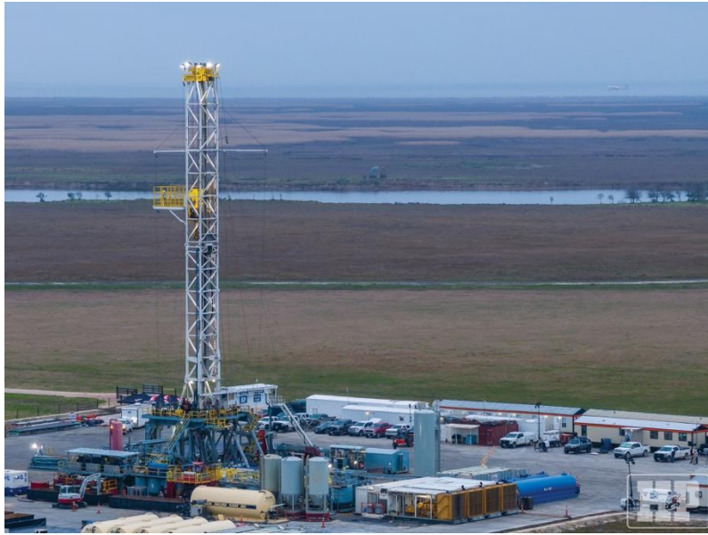
Figure 1: Representative drilling rig with similar specifications to the H&P 648 (FlexRigs®) planned for use in Omega's upcoming appraisal program. Vehicles located at the edge of the pad provide operation scale
