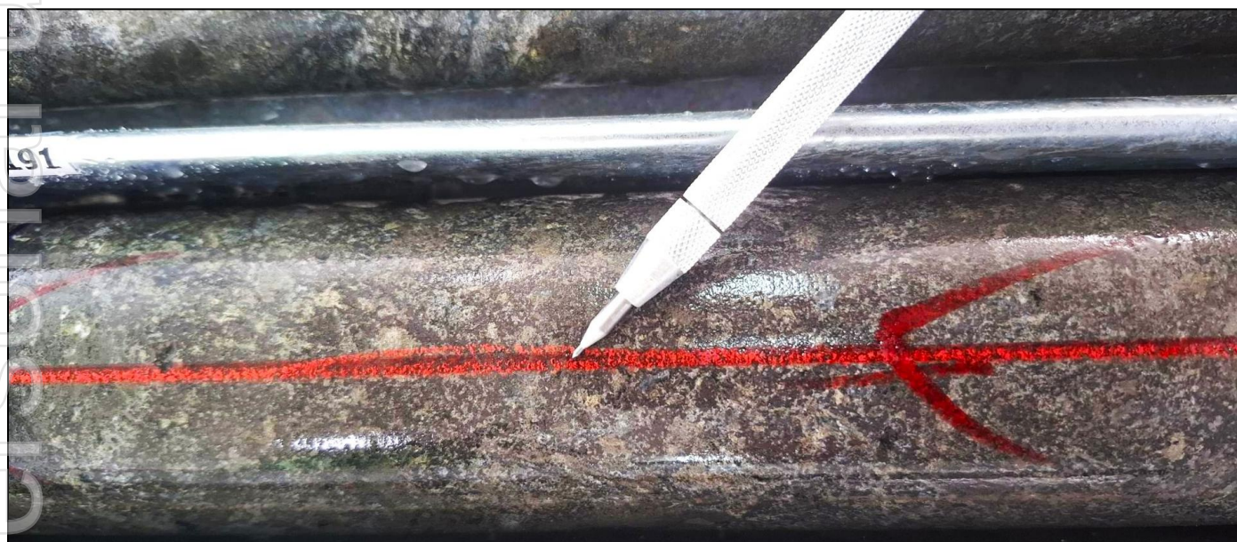
Figure 6. Core photograph from 333.7 to 335.7m in ZRSD25220 showing pyrite and sphalerite mineralisation – 4.3g/t Au, 8.9% Zn and 1.0g/t Ag.
