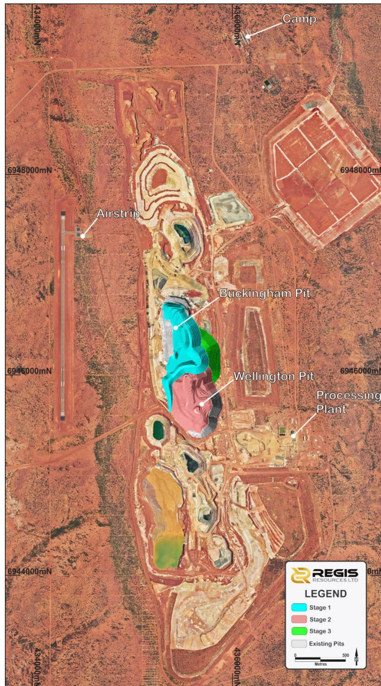
Figure 1: Buckingham-Wellington Open Pit cutback shown in three stages
