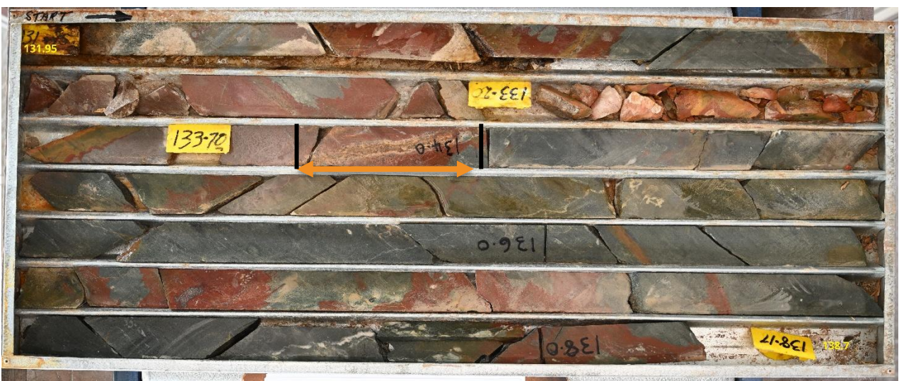
Figure 9: Mt Solitary - MS32 131.95 – 138.17m including (assay 131.95-134.0m 7.7g/t Au) hosted in epithermal veins (orange arrow) within a broad zone of increased chlorite and silica alteration and elevated iron oxides.
