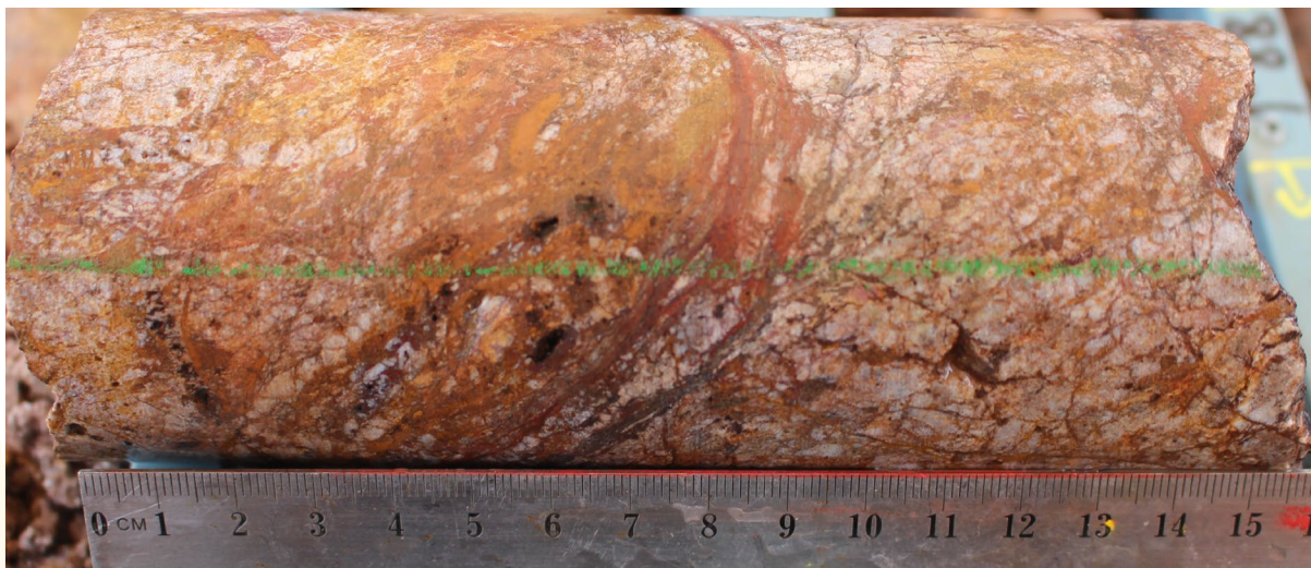
Figure 5 Selected drill core from Diamond hole at Seuss showing quartz breccia with quartz-hematite veining and possible weathered sulphides (HYDD25003 88.7-88.8m downhole depth)
