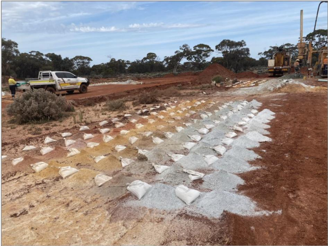
Figure 4. 1m samples from the RC drilling program.
