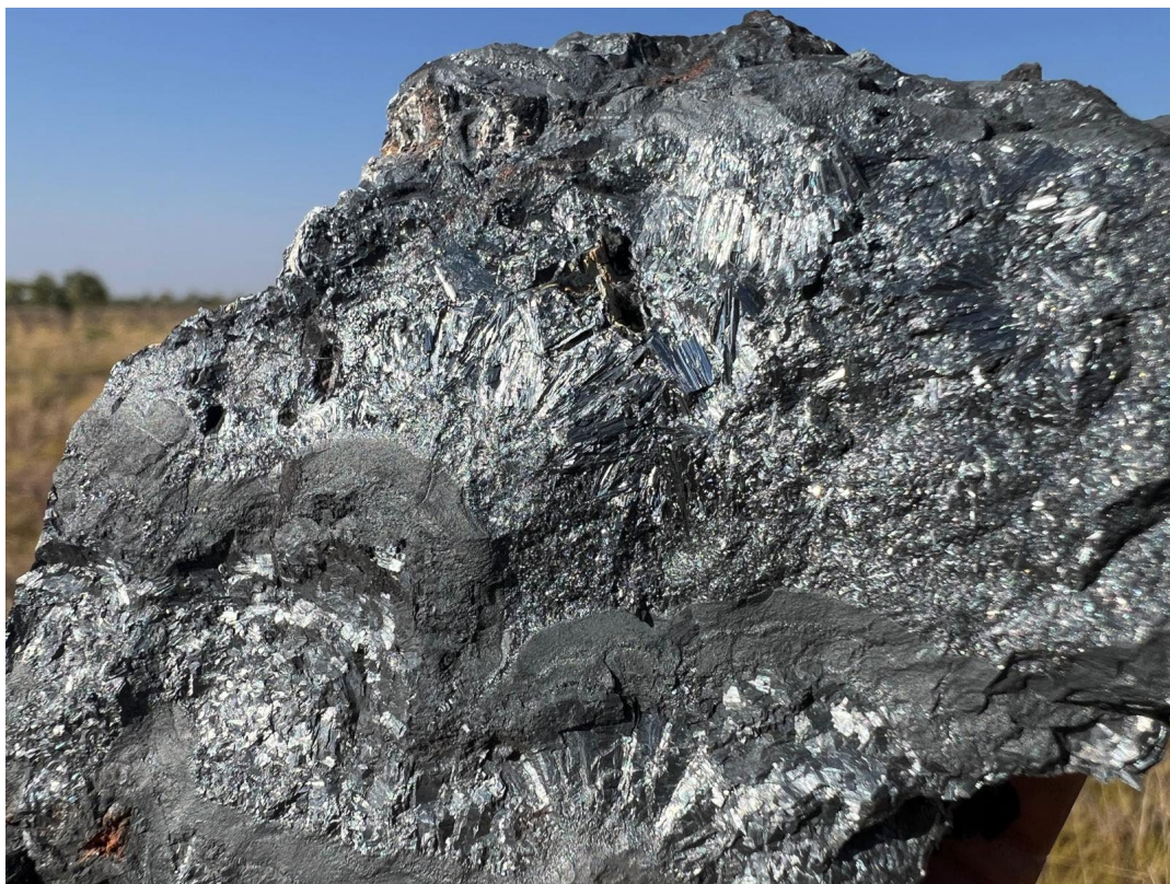
Figure 1. Stunning manganese outcrop rock chip sample photo showing interpreted near pure manganese oxide crystals at Trek's recent manganese discovery at the Christmas Creek Project (field of view 10cm).
