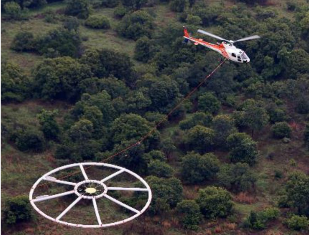
Figure 2. Xcite™ is a new generation of helicopter-borne time-domain electromagnetic (HTDEM) systems, developed by New Resolution Geophysics (NRG™), which can define conductive materials such as manganese oxides in mineral exploration.
