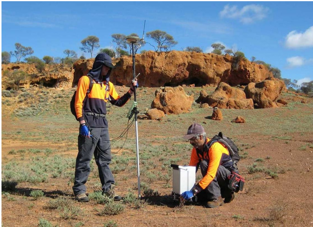
Figure 3. Atlas Geophysics specialises in ground-based gravity surveying. Processing and imaging of these measurements provides for the detection of subtle gravity changes due to lateral variation in sub-surface density. Due to the high density of manganese oxides in comparison to their surrounding host rocks, ground gravity is a suitable method to define an accumulation of manganese in the sub-surface.
