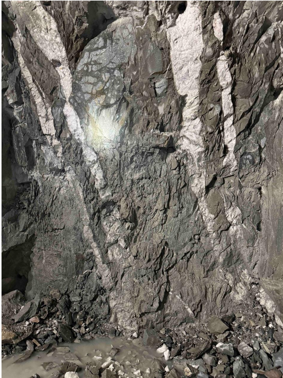
Figure 3 – 1600 Ore Drive showing multiple quartz veins in a 3m x 3m drive. Grade estimated at 4.2g/t.
