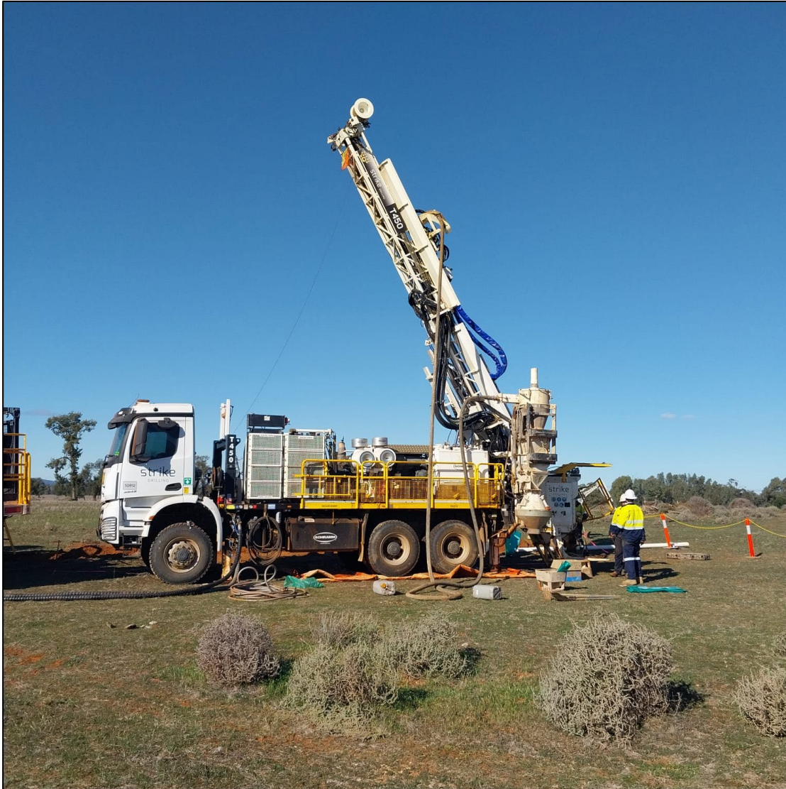
Figure 2: RC drill rig setting up on pad A2RC001 at the Road Base Quarry target. RC drilling is an air driven technique that smashes rock with a hammer, producing 30-40kg rock dust in a sample bag per metre.
