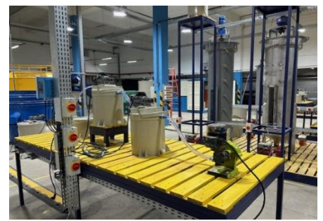
Figure 4 – Leaching circuit all plumbed up
