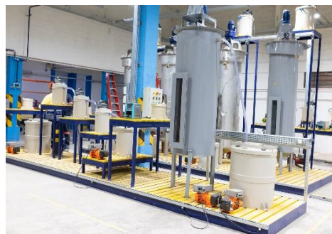
Figure 6 – Impurity Removal Circuit
