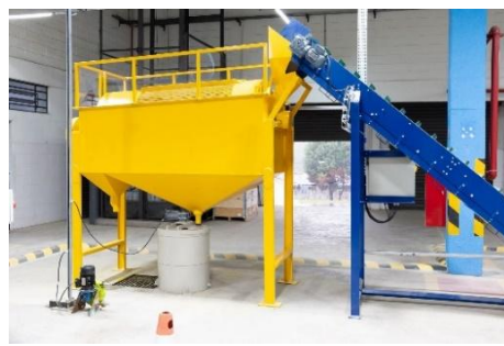
Figure 3 - Ore feed conveyor and scrubber
