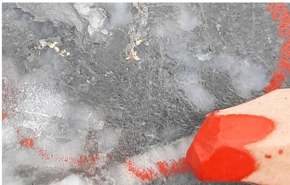
Figure 1. Multiple patches of visible gold 1 up to 2.5mm (lustrous yellow) within an irregular quartz stockwork zone in hole AMD014A at 466.0m. This interval graded 0.8 metres at 62.3g/t Au from 465.6m.
