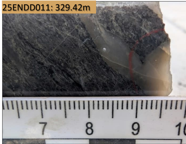
Photo 1. Visible gold (circled red) in hole 25ENDD011 at 329.42m down hole in quartz vein within granite host rock. Scale bar units are centimetres.
