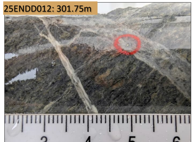
Photo 4. Visible gold (circled red) in hole 25ENDD012 at 301.75m down hole in quartz-carbonate-sulphide vein breccia within moderately phyllic altered granite host rock. Scale bar units are centimetres.
