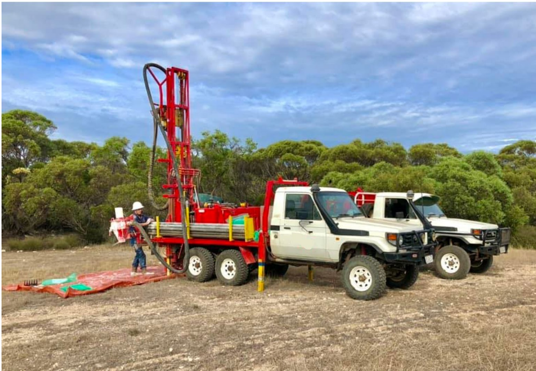
Figure 2. Typical 4WD mounted air core drilling rig.
