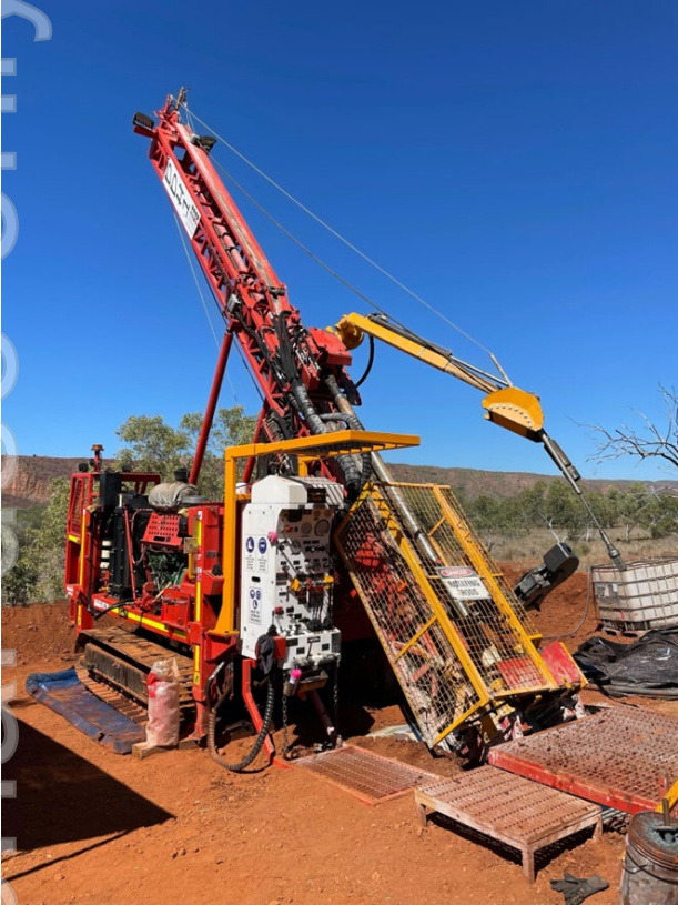
Figure 2: Track mounted diamond drill rig at Speewah site (left)
