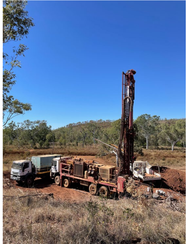
Figure 2: Track mounted diamond drill rig at Speewah site (left)
