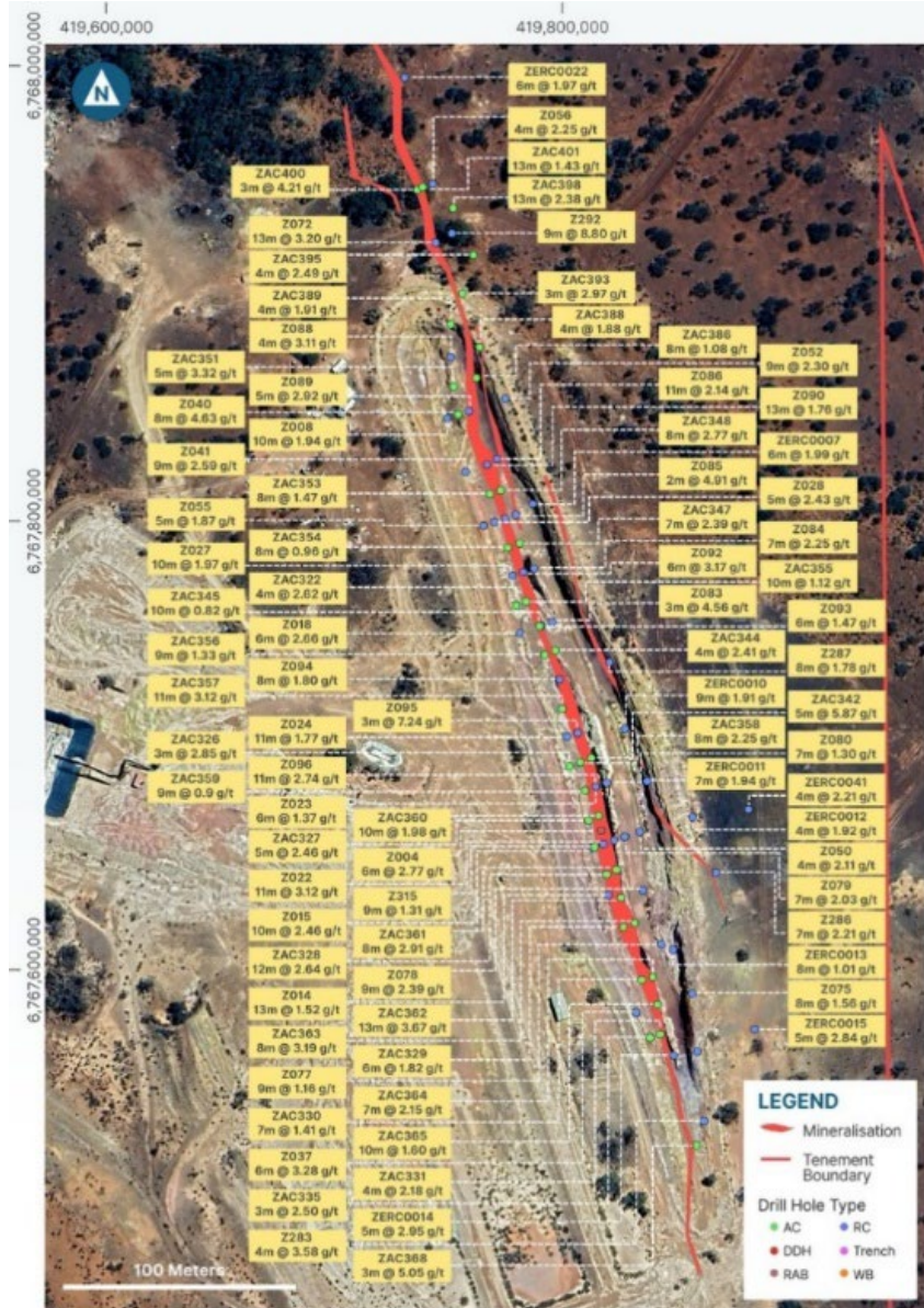
Figure 4: Aerial Photo of Zelica Trial Pit with Drilling and Projection of the Gold Mineralisation along approximately 300m of the ~1km mineralised strike 2
