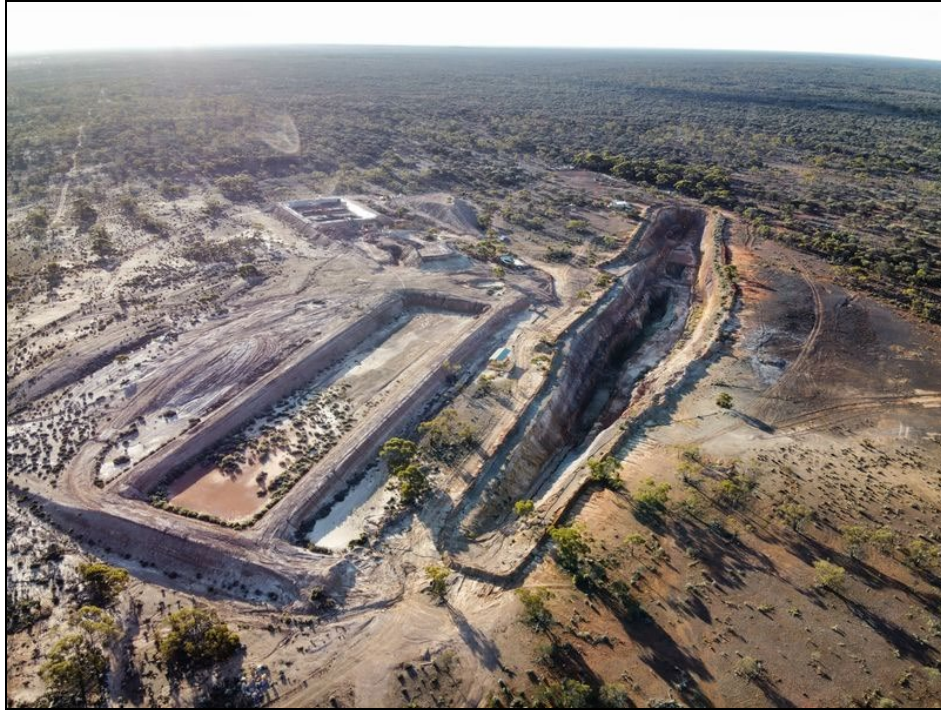
Figure 3: Drone photo of Zelica Project looking NNW showing pre-stripped open pit (approx. 300m long and 10-25m deep) and pre-constructed vat leach ponds (pic taken August 2025)
