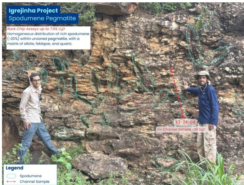
Figure 6– Outcropping spodumene-bearing pegmatite at Morro Grande (within the Igrejinha License 830851/2010), which contains individual spodumene crystals up to 50cm in size. Channel sample K2-24-04 also shown, which assayed at 3.26% Li 2 O. 11
