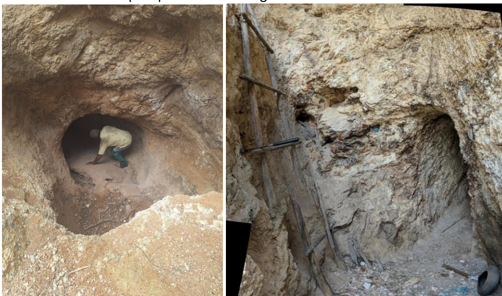
Figure 7: Artisanal mines identified at the Renaldinho prospect area, which are providing significant sub-surface mapping and sampling locations which are expected to aid in drill location targeting.
