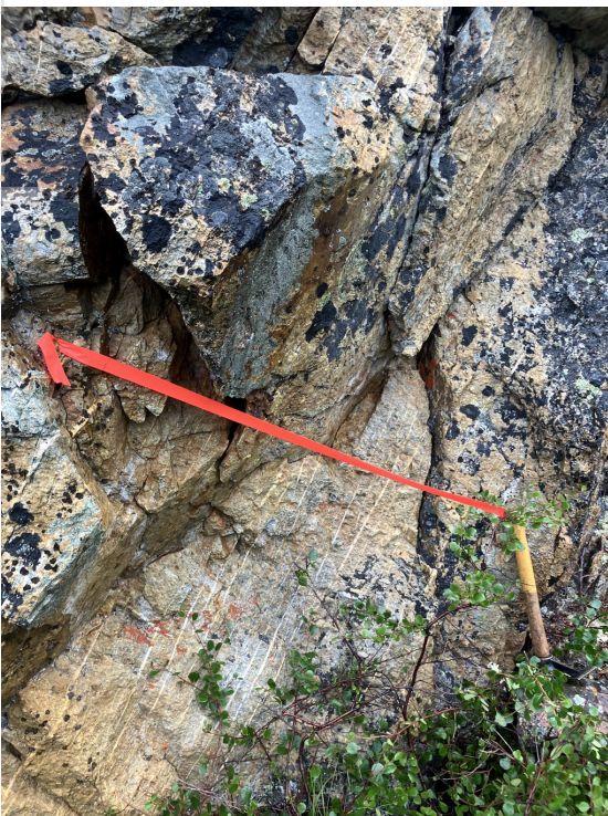
Figure 7: Field photo for sample G792106 of sheeted veins through sediments assaying 1.07 g/t Ag, 978 ppm As
