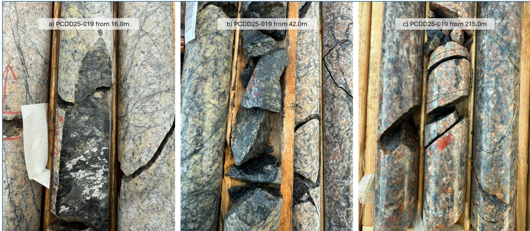
Figure 3: Drill core from PCDD25-019 (470813E, 5558967N, UTM Zone 21) demonstrating uraninite mineralisation in fractures.
