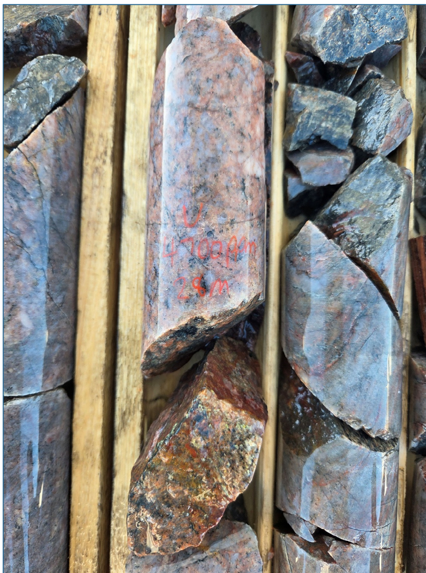
Figure 1: Visible uranium observed in PCDD25-014 (470462E, 5558025N, UTM Zone 21) at a drillhole depth of 28.0m.
