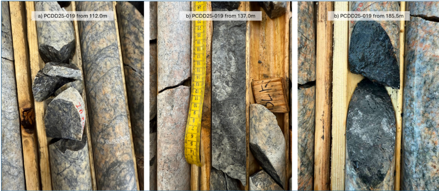
Figure 5: Drill core from PCDD25-019 (470813E, 5558967N, UTM Zone 21) demonstrating significant mineralisation of Zn, Cu and Mo in fractures.
