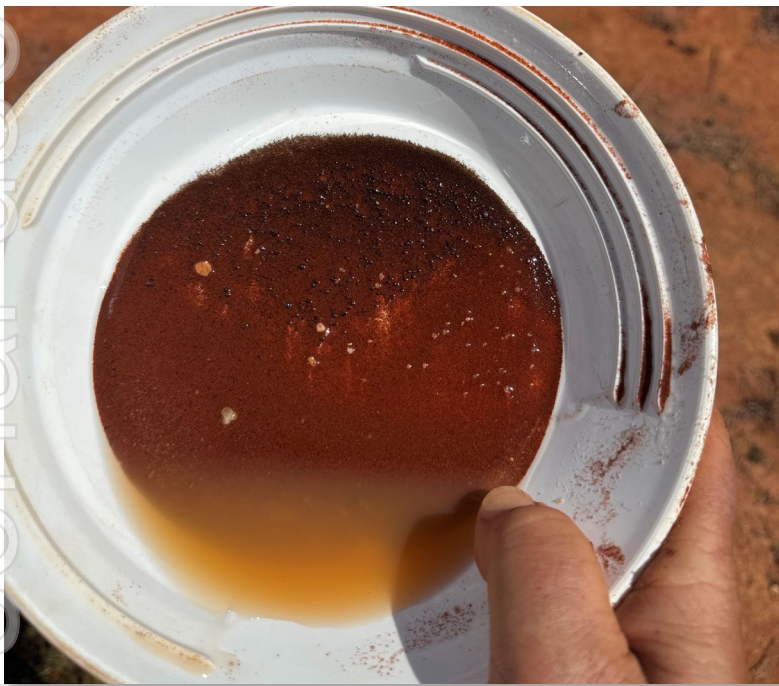
Figure 3: Typical pan-concentrated Heavy Mineral Sands (HMS) sample, Central EL6580 tenement, Irria Prospect.
