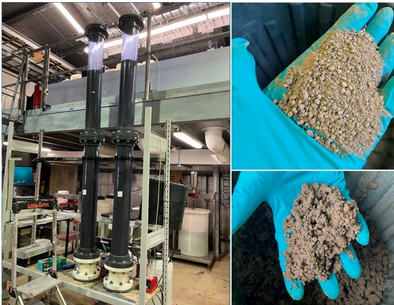
Figure 3: (a) ANSTO Facilities, Column C1 and C2 at 2m height, and displaying positive agglomeration and 'heaping' characteristics and showing REE mineralised sample (b) before agglomeration and (c) after agglomeration.
