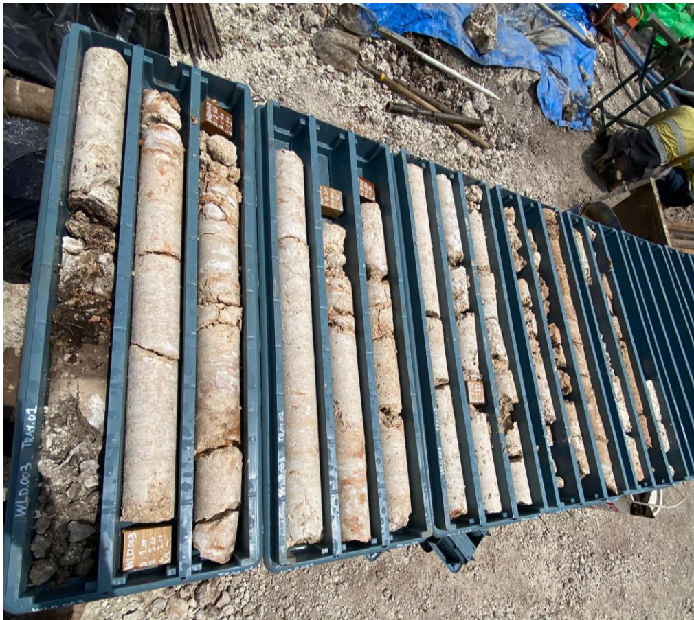
Figure 5: WLD003 drill-core from surface to approximately 15m, comprised of units of the Baucau Limestone (estimated 60% - 80% calcite). Assays are expected within 4-6 weeks. Refer to Cautionary statement above regarding Visual Estimates.
