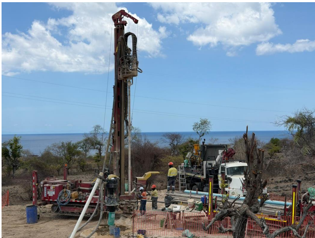
Figure 3: RC drilling in progress at the Werumata Limestone prospect.
