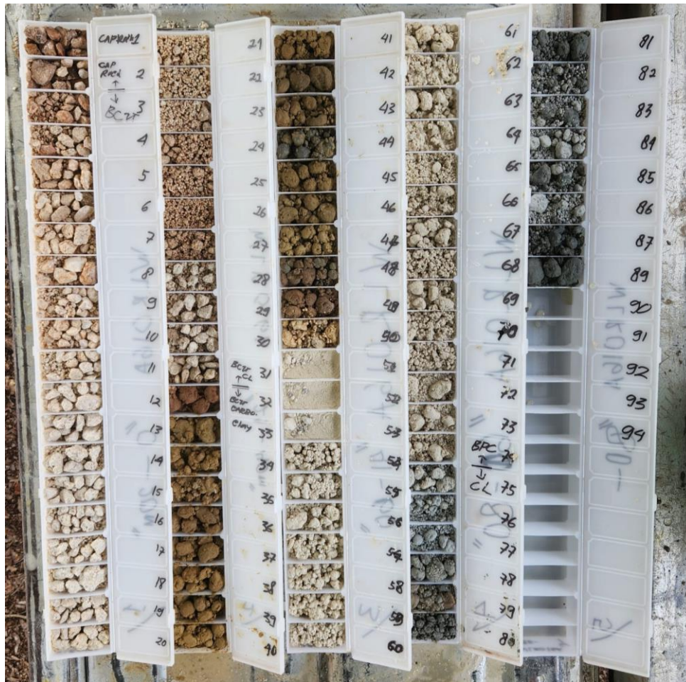
Figure 4: Chiptrays from drill-hole WLR016A; Baucau Limestone 0m – 31m (estimated 60% - 80% calcite) and Batu Putih Chalk 50m – 74m (estimated > 90% calcite). Assays expected within 4-6 weeks.
