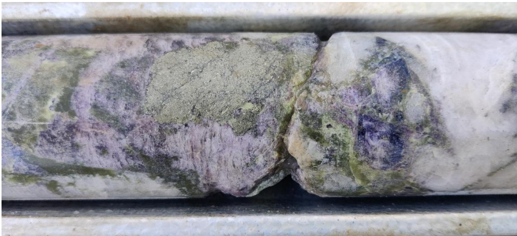
Figure 7: Intergrowths of Pyrite (metallic yellow, ~30%), Quartz (white, ~60%) and Fluorite (purple, ~10%) (IV001, 154.4m)
