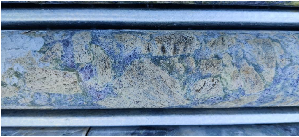
Figure 4: Carbonatite Alteration Textures Showing Intergrowths of Siderite (buff brown, ~70%), Calcite (white, ~10%) and Magnetite/ hematite groundmass (grey, ~30%) (IV001, 164.7m)
