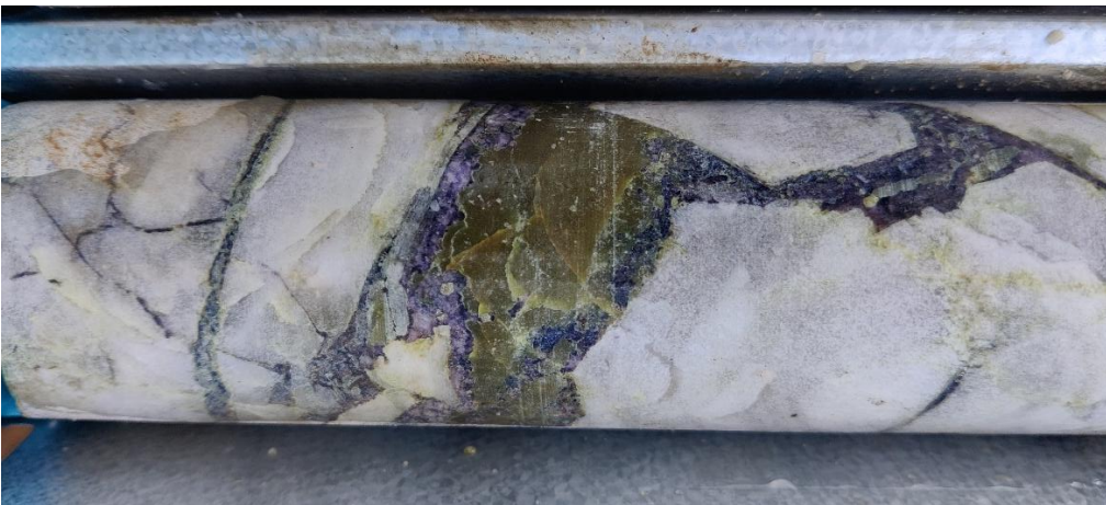
Figure 5: Evolved Fluorine-rich Mineralisation Comprising Breccia-like Fill of Fluorite (purple, ~10%) Topaz (green, ~10%) and Quartz (white, ~80%) (IV001, 152m)
