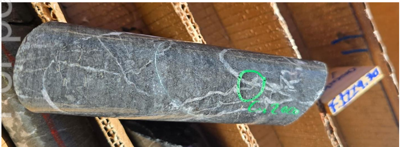
Photo 3. Anastomosing (cracked) textured veining and accessory sulphides at 1230m downhole in 25LLDD0070*.
