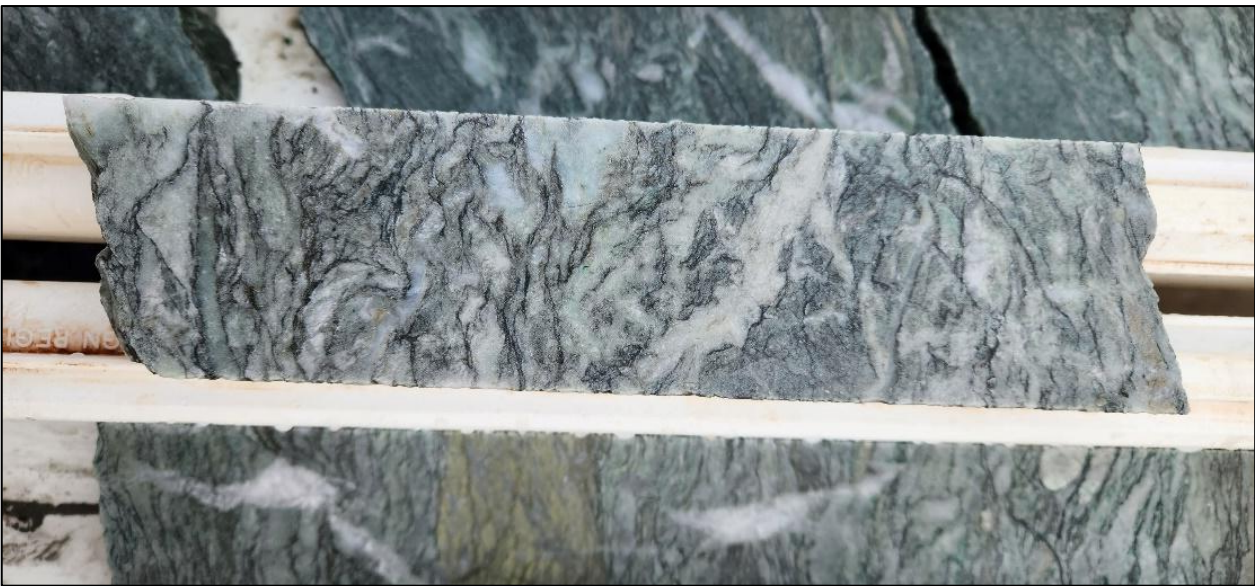
MLJDD019_148.4m_visceral texture in bleached, silicified ultramafic.
