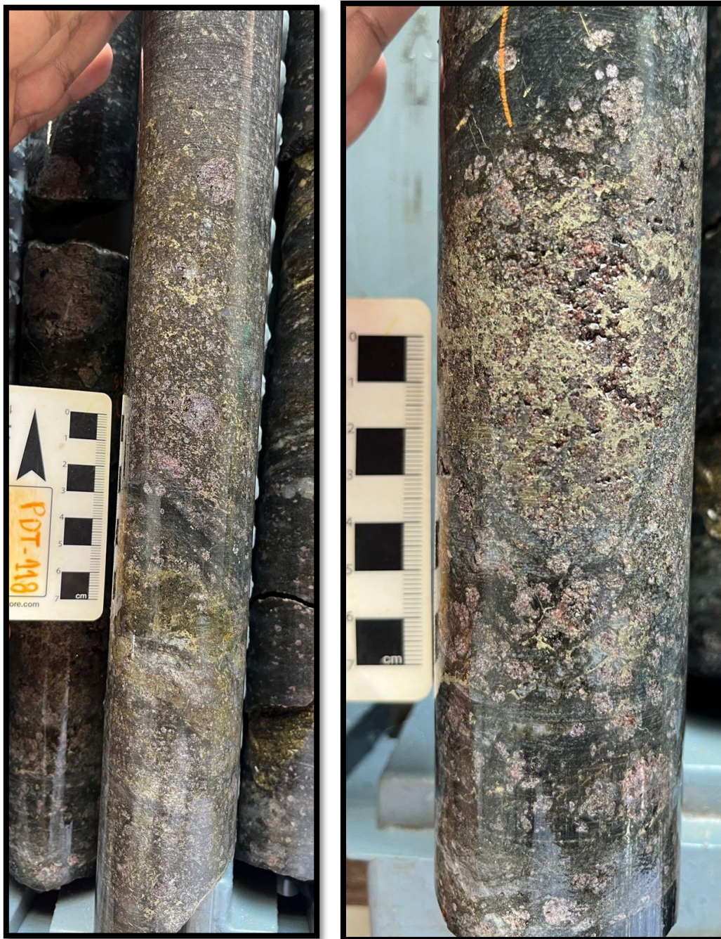
Figure 4: Mineralised intervals at Touro Prospect. From left to right: PDT-118 from 114.55m downhole and PDT-118 from 115.30m downhole. Depth refers to base of core in photo. Dark brown mineral is sphalerite (zinc sulphide), golden colour is chalcopyrite (copper sulphide), pale yellow is pyrite (iron sulphide) and bronze colour is pyrrhotite (iron sulphide).
