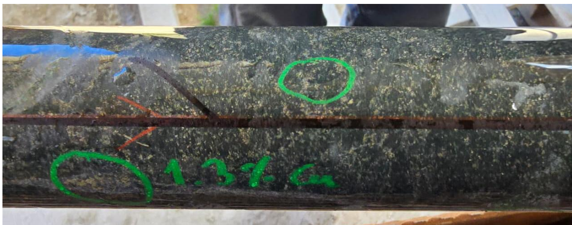
Photo 1. Disseminated sulphide mineralisation from a zone at 1268 to 1276.5m downhole in 25LHDD070* (refer to Appendix 1).
