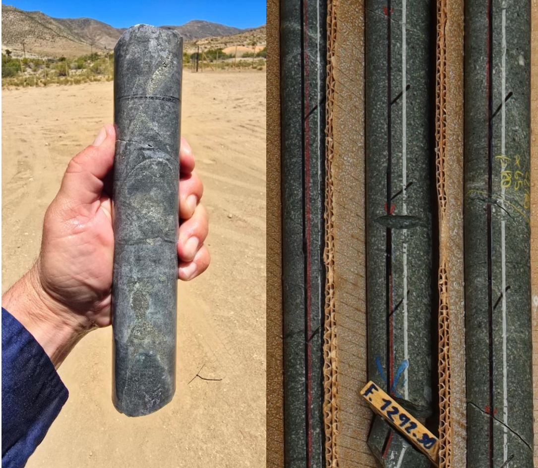
Photo 4. Strongly altered and mineralised (pyrite) core from 1283m downhole in 25LHDD070, immediately above the interpreted andesitic sill contact (left). Andesitic sill from approximately 1292m downhole (right).
