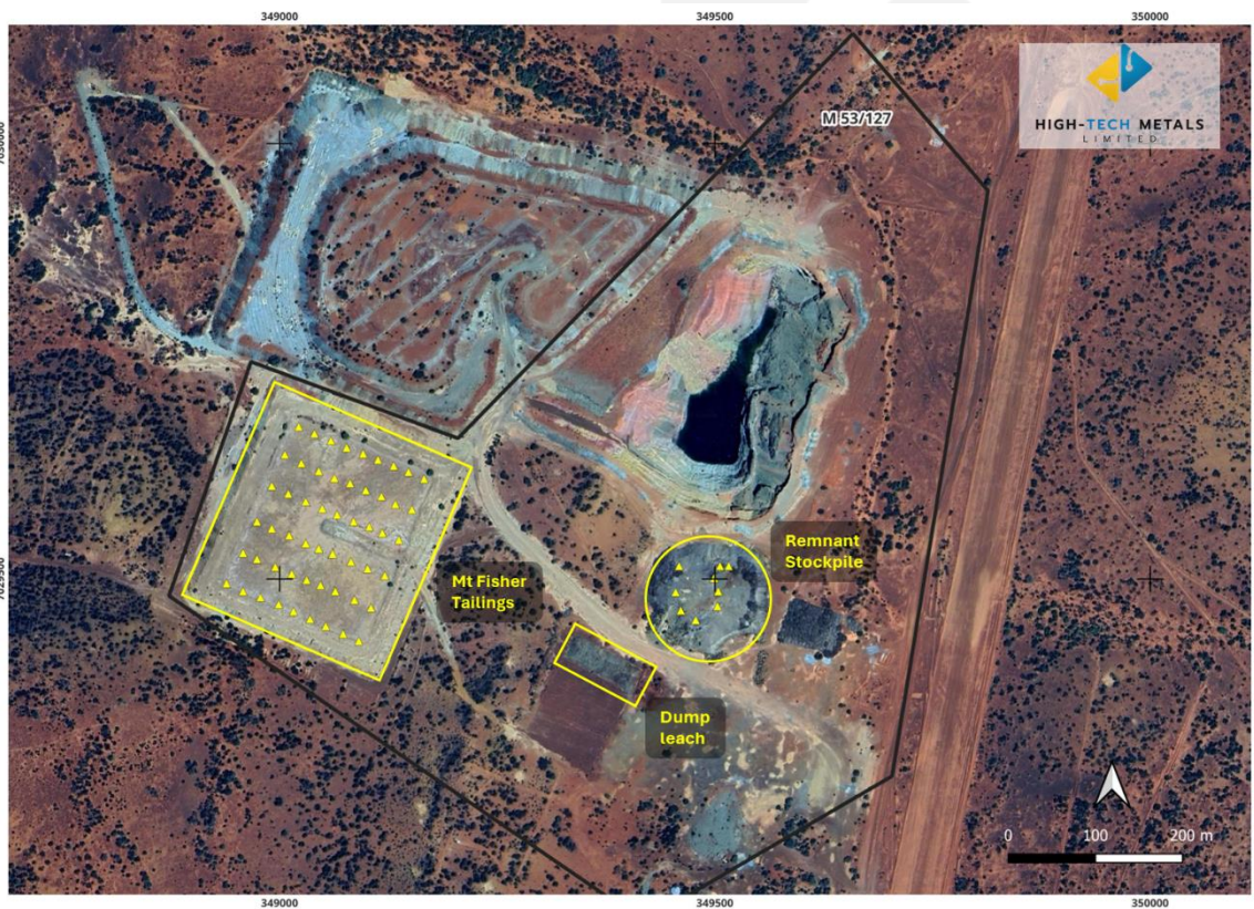
Figure 2: Mt Fisher (M53/127), 2025 metallurgical drilling and composite sampling program September 2025 (collars yellow triangles).
